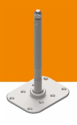
Using the BKS assembly kit post from INNOTECH, only a stop shaft is required for securing all further components in the horizontal lifeline system. The economical BKS assembly kit post is made up of two components, and is used in the lifeline system as a single anchor point or as an end, corner, and intermediate post. In addition, it can also be used together with INNOTECH SPAR-10-25 as a single anchor point.
