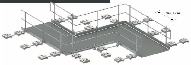
The SYSTEM-VARIO escape route from INNOTECH is held by self supporting load and therefore installed without roof perforation. The width of the flexible system is adjustable, requires significantly less material because of the greater separation distances, and therefore reduces the superimposed load.
